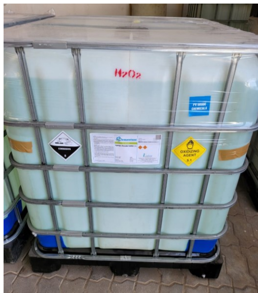
Figure 1: Hydrogen Peroxide PV grade ready for transport in an IBC with proper labeling. As shown above, brown taping is used for easy visual identification. All KOH IBCs at our facility are stored together to maintain compatibility.
