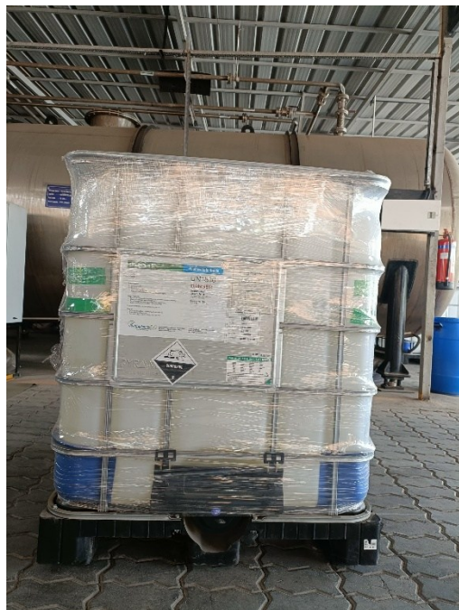
Figure 1: Sulfuric Acid PV grade ready for transport in an IBC with proper labeling. As shown above, green taping is used for easy visual identification. All H 2 SO 4 IBCs at our facility are stored together to maintain compatibility.
