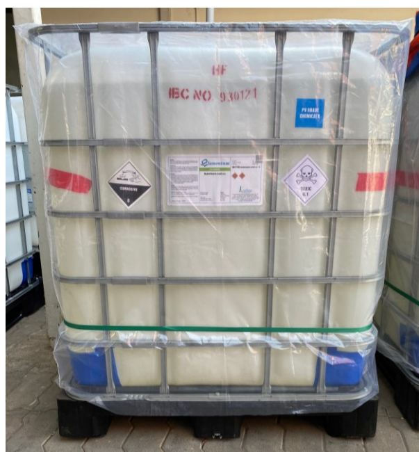
Figure 1: Hydrofluoric Acid (HF) PV Grade stored in compatible IBCs and properly labeled with pictograms and the company's customized label.
