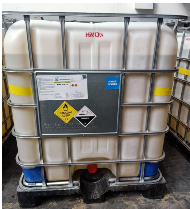
Figure 1: Nitric Acid (HNO 3 ) PV / EL grade stored in an IBC with proper labeling. As shown in the above image, use of color coding is incorporated for easy visual identification (yellow taping for HNO 3 ). All HNO 3 IBCs at our facility are stored together to maintain compatibility.
